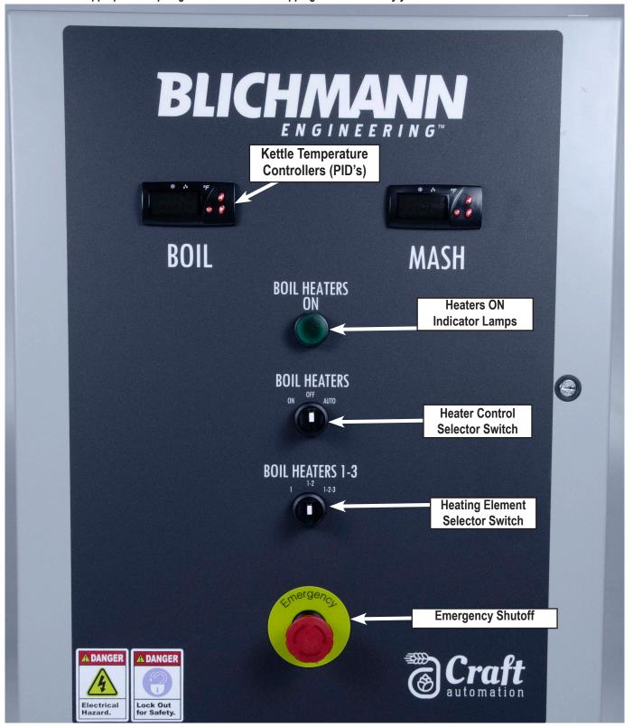
Panel pictured is a single phase controller. Locations of the components in the three phase panel will be the same.
