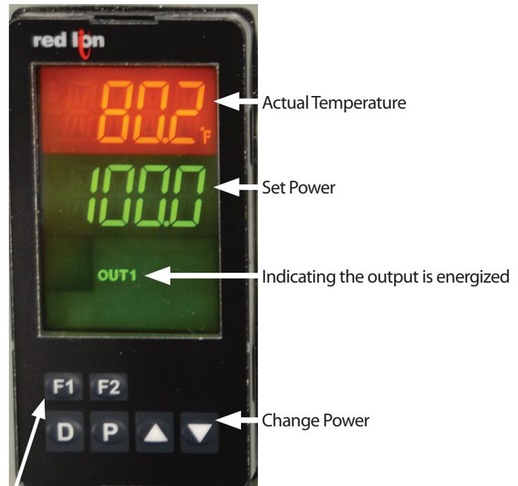
Switch between temp control and power control
