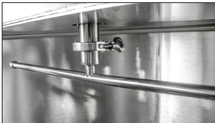
**IMPORTANT:** Do NOT sparge or vorlauf at full pump flow or you are very likely to stick your mash, and your efficiency will suffer severely!
