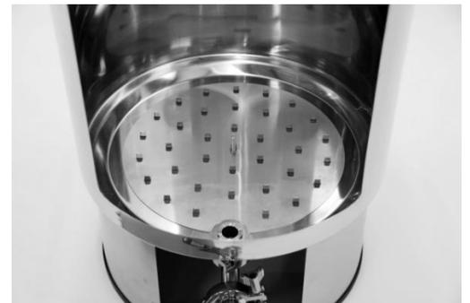
**Important:** The tabs must face upward! Installing the tabs downward will block off most of the perforated screen causing the press to malfunction!
