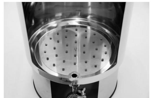
Install the screw-eye in the false bottom as shown. This is used as a handle to remove the false bottom after use, and then place it on the bottom of the fermentor. Use the large fender washer and wing nut to secure it to the bottom of the fermentor. Finger tight is plenty – do not over tighten.
