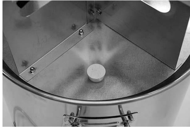
Tighten guide bars in this position ensuring piston is level
