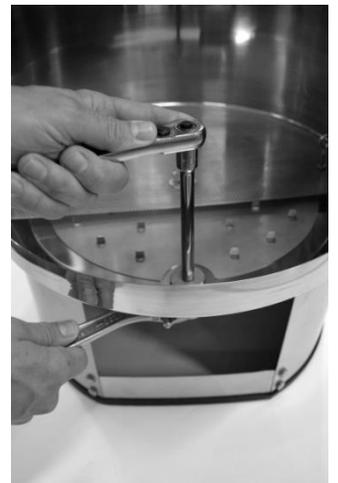
wrench on the outside. Do NOT use Teflon tape on these threads! Note that the wrenches are not supplied.
