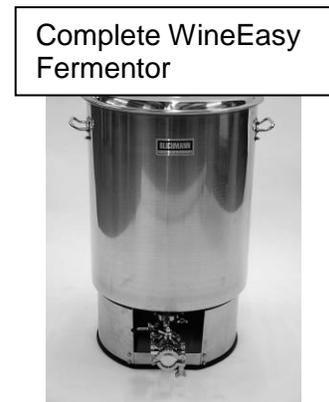
**IMPORTANT:** Prior to assembling the fermentor it is important to ensure that the tank has not been bent from shipping. Use a tape measure to check for circularity – the difference in inside diameter all around the tank should be less than 1/8". If it is slightly out of round, simply lay the fermentor on its side and push gently to reshape it. Otherwise contact your retailer.
