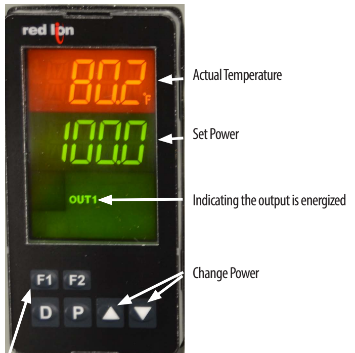
Switch between temp control and power control
