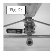
**Caution**: If you use use wrenches to tighten the o-ring fitting on the bottom dump do not over-tighten or you may damage the tank or the fitting. A snug fit is all that is needed to get a good seal.
