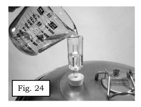
**Important:** Dry the outside of the tank with a cloth and if any fittings are leaking, tighten them as required, taking care not to bend the tank. If you are unable to resolve a leak problem please re-read the fitting assembly instruction thoroughly taking special note of the location of the o-rings and retainers. If you are still experiencing a leak, contact Blichmann Engineering as this is not normal.
