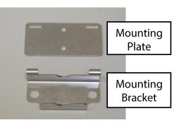
Assembly is quite simple. Place the 1/4" bolts through the mounting plate and LTE stand. Secure with the 1/4" nut (Fig. 1). Mount the chiller to the mounting bracket using the mounting studs on the chiller and the nuts included with the chiller as shown in Fig. 2. Set the mounting bracket into the mounting plate slots as shown in Fig. 3.
