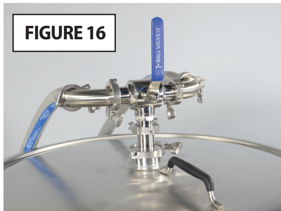
T-shaped three-way valve on top of the mash tun allows the flexibility to bypass the mash tun kettle or it can be turned for sparging or CIP (Clean-In-Place).
