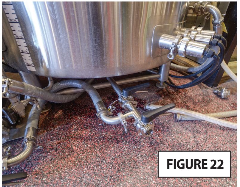
Please note that the hoses are tucked under to allow ease of portability, this reduces tripping hazards.
