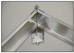
Attach the lifting arm to the holes in the mash kettle strand. Use the included allen wrench to tighten in place.
