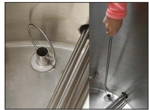
Install the false bottom through the manway in the mash tun (MT) one segment at a time starting with the center section. Install the U-shaped securing clips between the sections to secure them as shown.
