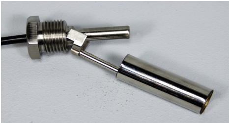
Picture shows float switch down. In this position the heating elements will not energize.
