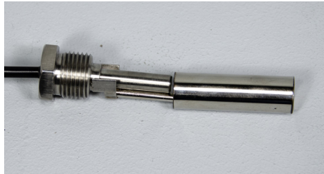
Picture shows float switch up. In this position the heating elements will energize.
