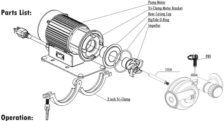
Connect the pump to your system using heavy wall and/or braided hoses. It is highly recommended to use  $\frac{1}{2}$ " ID x .125" wall silicone tubing. This hose will handle the pressures and temperatures of the beer brewing processes. Secure all hoses with clamps.
