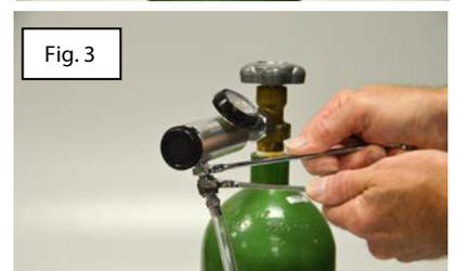
**CAUTION** – take care not to twist the fitting on the regulator or the fitting may be permanently damaged. This is not a warrantable failure.
