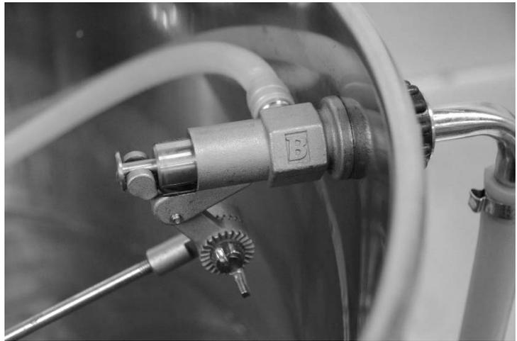
**Heat to Strike Temperature:** Open all valves fully and then turn on your pump. Add any water salts and acids at this time. Turn on your heat source until you reach your desired strike temperature. At this time close all valves and turn off the pump.
